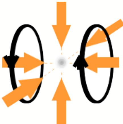
Figure 3: Principle of the magneto-optical trap (MOT). The MOT consists of three pairs of counter-propagating beams with opposite  $\sigma^+/\sigma^-$  polarisation plus a pair of coils with opposite current for the magnetic field gradient.
